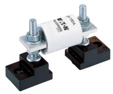
The simpler design is the C5268 modular fuse block. With this design, the fuse terminal and cable (with termination) are mounted on the same stud, minimizing installation labor. The stud type block is available in the configurations shown in the table below.
