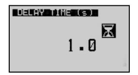
A "delay before response can be set for relays. The screen below will be displayed after first two steps. Set the required delay time here.
