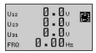
The unit checks continuously the sequence of AC phase voltages.
