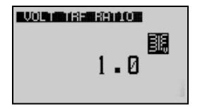
If a voltage transformer is used, then its ratio needs to be set to the unit.
