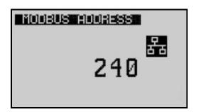
Select "MODBUS ADDRESS" on "CONFIGURATION MENU". Change the modbus
