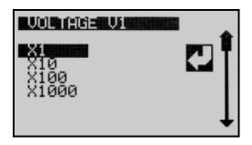
After selection of the item, the limit value should be entered. Especially for power or user counters, large values may be needed. Thus the user must select the multiplier first ('x1','x100' or 'x1000').
