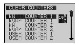
The unit offers 2 sets of active and reactive power counters together with 4 user counters. Counters can be reset via the configuration menu whenever required.
