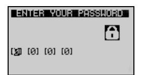
When the configuration mode is entered, the password entry screen will be displayed.
