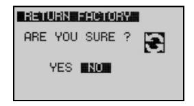
It is possible to reset the unit to factory settings, before starting a new configuration process.
