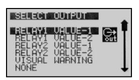
After entering the limit value of the item, the action to be taken when the condition occurs has to be selected.
