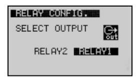
The unit has 2 relay outputs with configurable functions.
