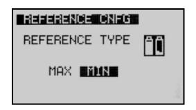
Select "REFERENCE CNFG" on "CONFIGURATION MENU". Select low limit (minimum acceptable value) or high limit (maximum acceptable value) of the item to
