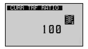
For the correct current measurement, the current transformer ratio has to be set properly.
