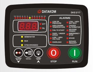
The fault conditions are considered in 2 categories as Warnings and Alarms. Measured values have separate programmable limits for warning and alarm conditions.
