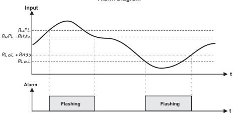
When an alarm occurs, measured temperature value flashes on display.
