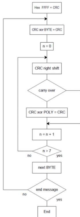
**CRC CALCULATION (CHECKSUM for RTU)**
